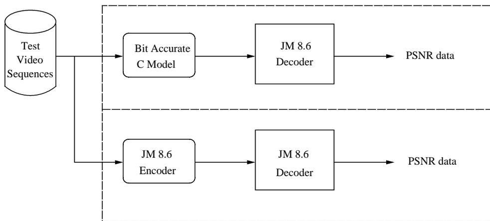
Each video sequence is encoded by the H264-E C model as well as the JM 8.6 H.264 software encoder reference model. The resulting bitstreams are decoded by the JM 8.6 H.264 software decoder. File size and PSNR information is then recorded and reported.
